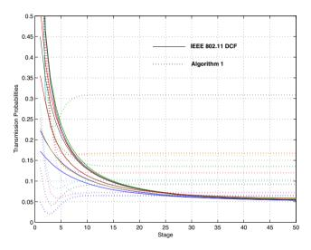
Fig. 13. Transmission probabilities of Algorithm 1 and the IEEE 802.11 DCF in ad-hoc networks.
