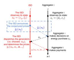
Fig. 3. Illustration of the entities' decision making and information exchange. The action and the message exchange in the dashed box are related to the conjectured prices proposed in the design framework in Sec. IV.
