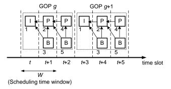
**Fig. 1** Illustration of GOP (group of pictures), DU (data unit), and the context. Since the scheduling time window is W = 2, the contexts in different time slots are  $C_t = \{DU_1^g, DU_2^g, DU_3^g\}$ ,  $C_{t+1} = \{DU_2^g, DU_3^g, DU_4^g, DU_5^g\}$ ,  $C_{t+2} = \{DU_4^g, DU_5^g, DU_1^{g+1}\}$ ,  $C_{t+3} = \{DU_1^{g+1}, DU_2^{g+1}, DU_3^{g+1}\}$ , and so on.
