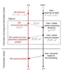
Fig. 2 Illustration of the interaction between the BS and user i (i.e. their decision making and information exchange) in one period.
